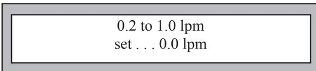
You may adjust the flow upwards by pressing the POWER switch (arrow up) or downwards by pressing the SELECT switch (arrow down). If you set the flow to 0.0 LPM, the instrument will disable the pump and enter the flow draw mode. **Please refer to section III. Normal Operation: Sample Draw Mode for more information.** If you set the flow between 0.2 and 1.0 LPM, the instrument will automatically adjust the pump to the requested flow rate using feedback from the built-in mass flow sensor.
