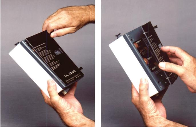
The cell is keyed to ensure proper alignment into the instrument. When installed, the circuit board of the cell should be flat with the bottom of the instrument. Push up on the clear window at the back of the instrument to eject the cell.
