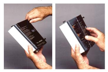
The cell is keyed to ensure proper alignment into the instrument. When installed, the circuit board of the cell should be flat with the bottom of the instrument. Push up on the clear window at the back of the instrument to eject the cell.
